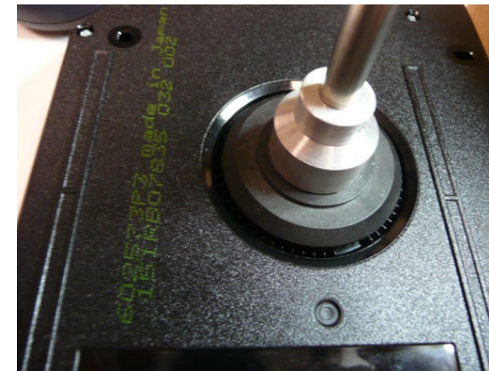
Figure 2. LTO and TS1150/TS1155 cartridge engagement designs are the same.
