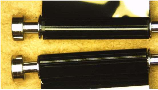
Figure 1. Leader Pin—LTO vs. IBM TS1150/TS1155
