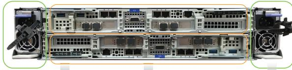
Dual-node server with two hot-swappable compute canisters. Each compute canister can access all 24 drives.
